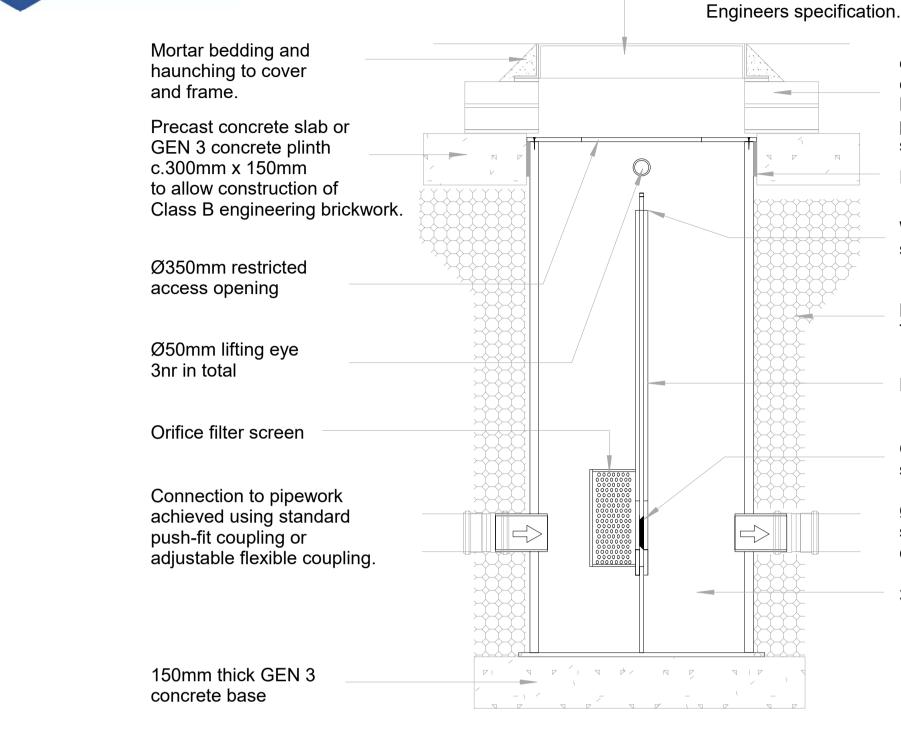
INSTALLATION DETAIL WASP06102WW Series Prefabricated Weir Wall Flow Control Chamber Ø600 up to 1.5m deep chamber By SEL Environmental Tel: 01254 589987
